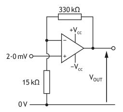
(a) Calculate the output voltage from the op-amp shown above.
