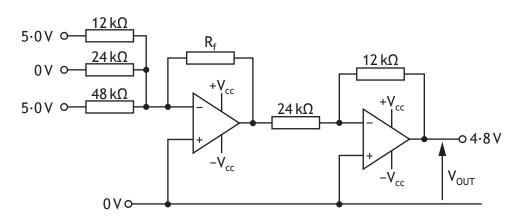
(f) Calculate the value of the feedback resistor,  $R_f$ , when  $V_{OUT}$  is 4.8 V.
