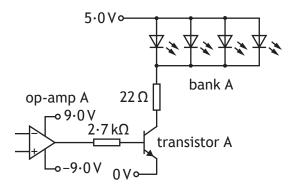
(b) (i) Calculate the base current for transistor A when op-amp A is saturated positive. (Assume  $V_{be}$  is 0.70 V).
