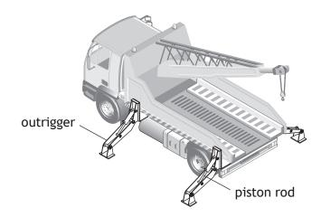
The piston in each outrigger produces a force of 49 kN. The piston rods are to be manufactured from mild steel with a factor of safety of 15. The piston rod has a circular cross section.
