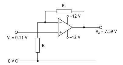
(a) Calculate the gain for this circuit when the input voltage is 0.11 V.
