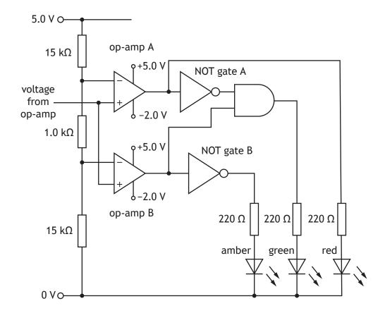
An amber LED lights if there is not enough material. A green LED lights if there is the correct amount of material. A red LED lights if there is too much material. When the op-amps saturate negatively they will output 0 V.
