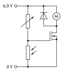
(c) Calculate the drain-source current when the MOSFET is fully saturated.
