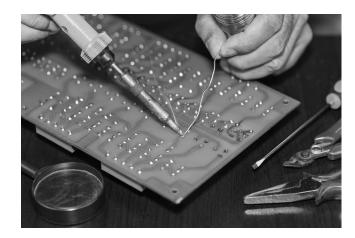
The soldering iron uses a two-state control system to turn the heating element on and off, and to monitor its output to maintain the desired temperature.
