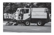
The street sweeper makes use of various rotating brushes which collect dirt and debris. Each brush is connected to a plate which is driven by a motor shaft as shown below.
