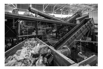
One stage of the process uses weight sensors to detect plastic waste. Jets of air from a fan are then used to separate the plastic waste from heavier items such as metal waste.
