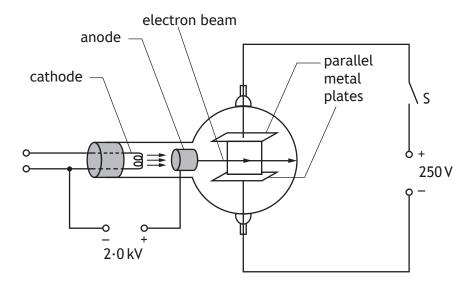
(a) Electrons are accelerated from rest between the cathode and the anode by a potential difference of  $2.0 \, \text{kV}$ .
