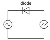
Current can only flow in one direction through a diode.
