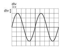
The Y-gain setting on the oscilloscope is 2.0 V/div.
