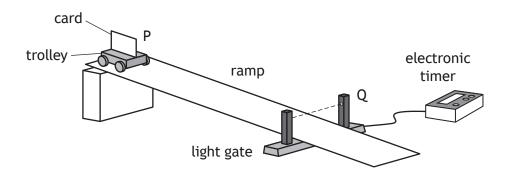
The trolley is released from rest at point P and moves down the ramp.
