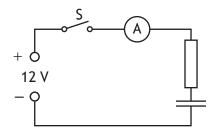
The capacitor is initially uncharged.
