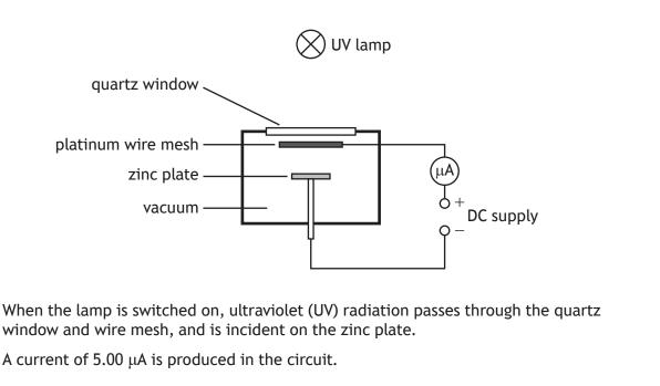
(a) (i) The lamp emits UV radiation with a frequency of 1.25 × 10<sup>15</sup> Hz.
