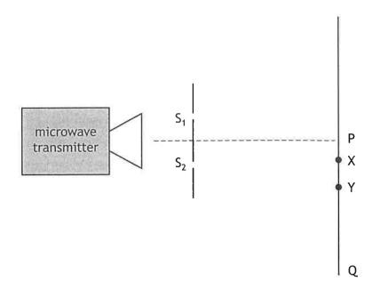
A radiation detector is moved along the line from P to Q.
