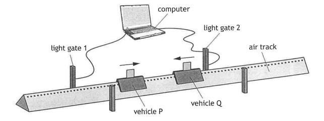
The mass of vehicle P is 0.18 kg and the mass of vehicle Q is 0.24 kg.
