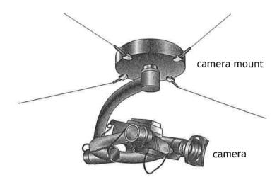
The camera mount is suspended from four cables. The length of the cables can be changed using a motor attached to each cable. This allows the height and position of the camera over the pitch to be changed.
