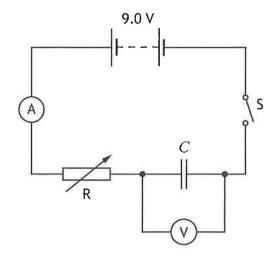
The resistance of the variable resistor can be adjusted to maintain a constant charging current.
