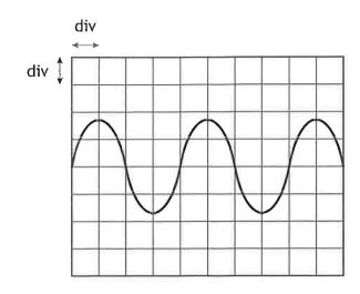
The timebase setting on the oscilloscope is 5.0 ms/div.
