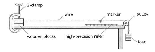
The student applies a force to the wire, which causes the wire to stretch.
